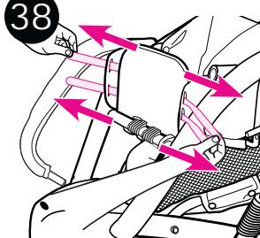
Thread straps through button holes on each side of seat cover.
